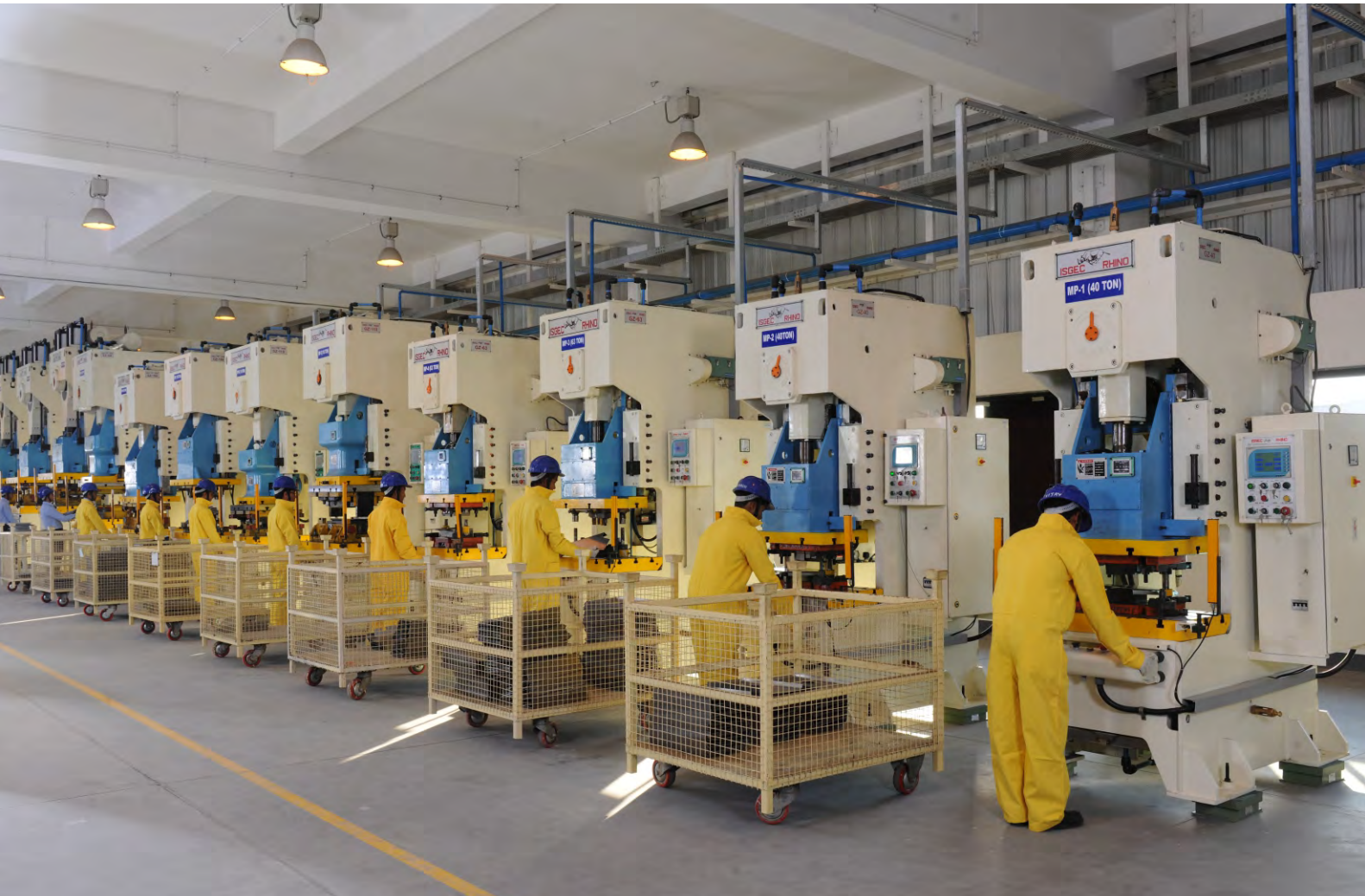
A battery of Presses (40 T to 300 T Capacity) supplied to MUSCO, India for production of components for Tata Motors.
