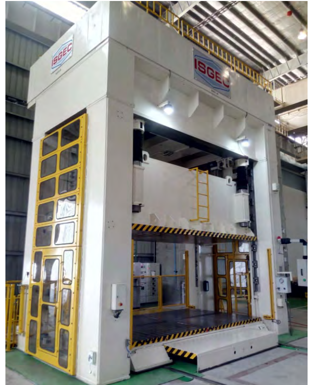
300T Die Spotting Press supplied to Japanese OEM in India
