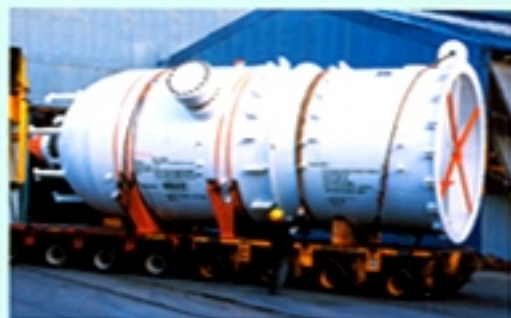
Mercury Adsorber Vessel, 157 mm thick, weighing 130 MT and ASME 'U2' Stamped, supplied to Petroleum Development, Oman.
