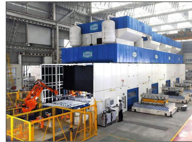
Transfer Press for Big Rapids Products, USA
