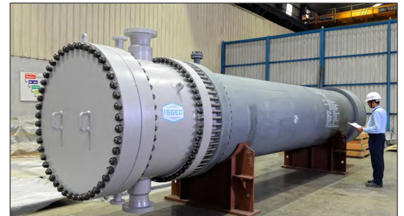
Helical Heat Exchanger for ExxonMobil, Thailand
