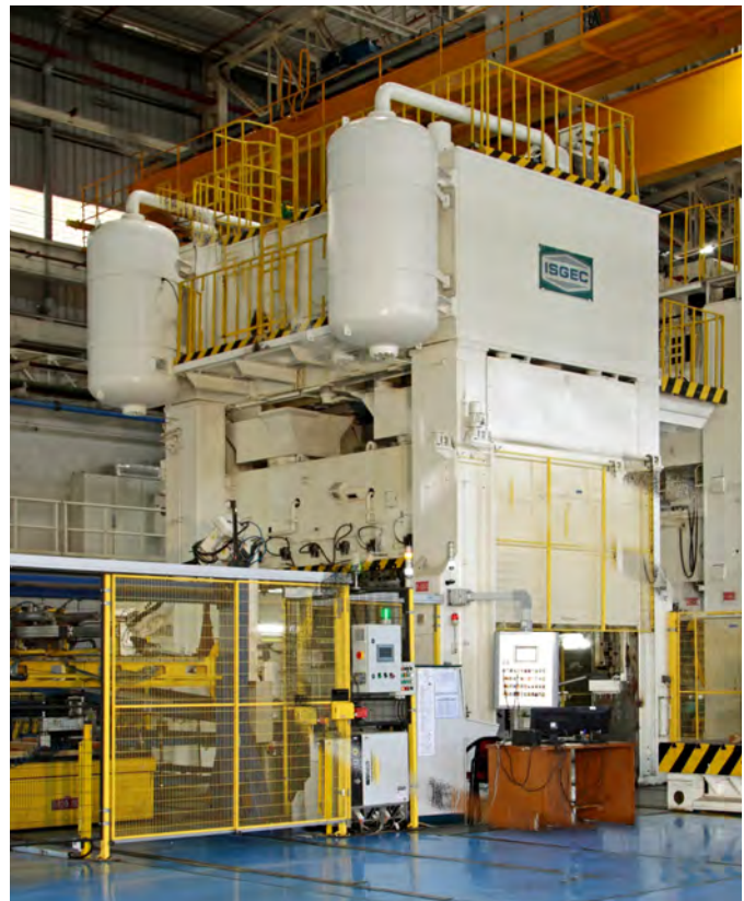
1200T Mechanical Press supplied to a Tier-1 Automobile Ancillary in Pune, India
