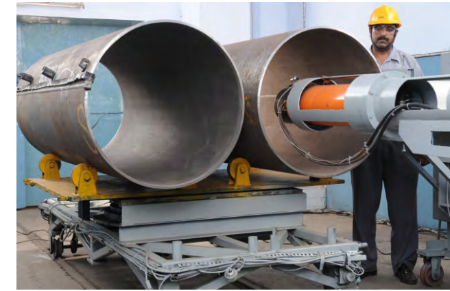
Such X-Rays further prove that all welds are sound. Today many of these are in digital form
