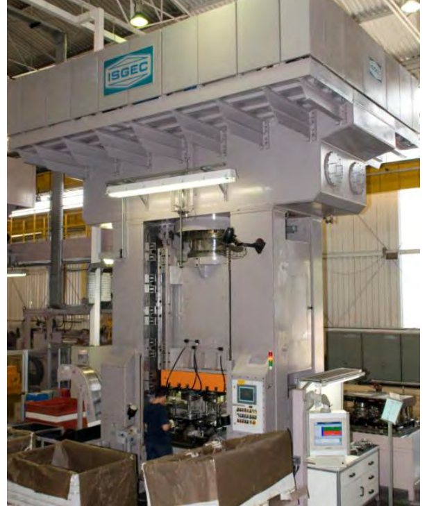
1500T Hi-speed Hydraulic Press supplied to a German MNC in Brazil for manufacturing Clutch Components. Similar supplies made to their plants in South Africa & India
