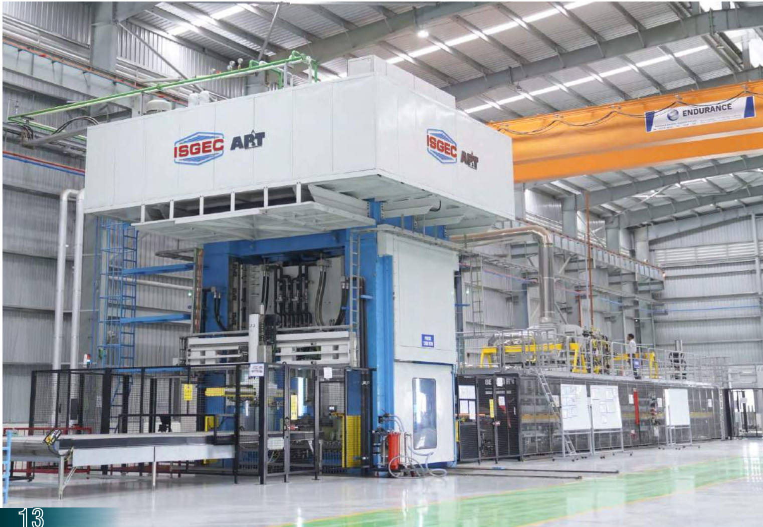
1200T Hydraulic Hot Forming Press at Tier-1 automobile supplier in India
