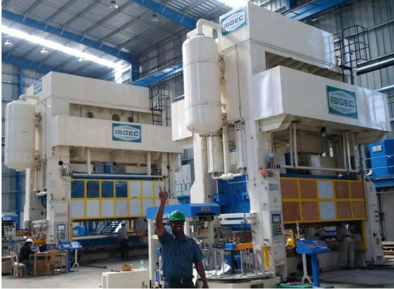
1250 T Transfer Press with Bolster Size of 4300 mm x 1400 mm & 630 T with Bolster Size of 3700 mm x 1400 mm integrated with Korean make transfer system supplied to Auto Tier-1, Bangalore, India supplying majorly to most 4 Wheeler & 2 Wheeler OEM's
