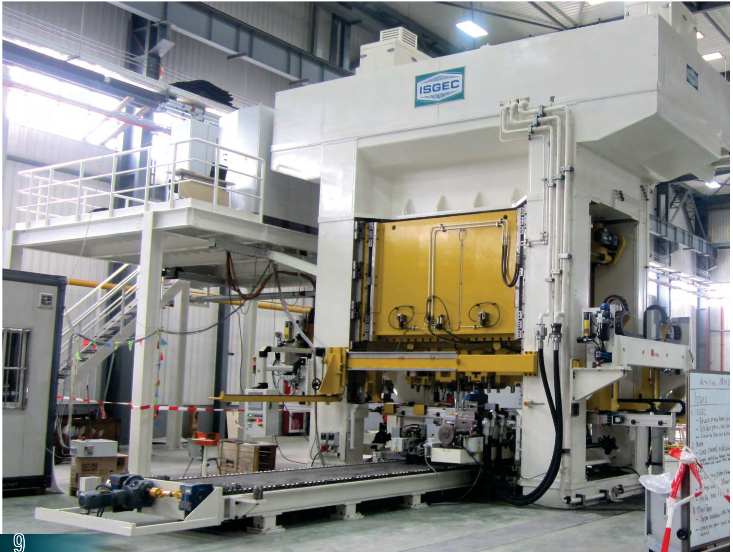
800 T Hydraulic Transfer Press with Parallelism Control System, supplied to German Multinational for their plant in Shanghai, China
