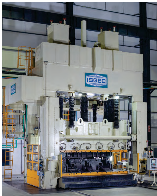
1000 T Tryout cum 300 T Die Spotting Press supplied to Japanese Stamping Dies manufacturer in India
