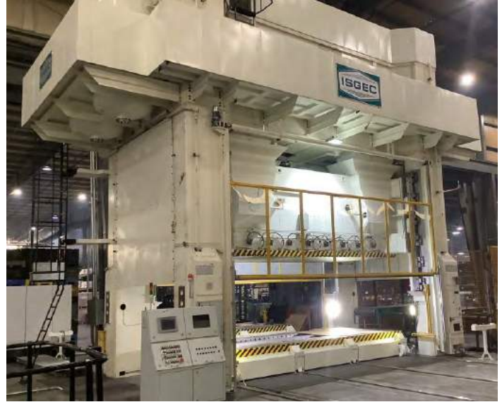
1500T Mechanical Transfer Press supplied to automobile seats manufacturer in USA for their plant in Mexico
