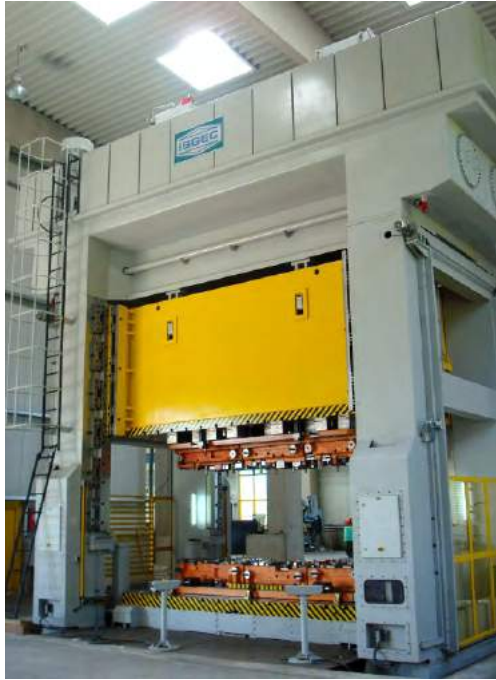
1200T Hydraulic Press was supplied in Germany for tryout and manufacturing critical components for Auto majors. The Press is equipped with moving bolster of size 4500 mm x 2200 mm and has provision for mounting Dampers, which makes it suitable for blanking.
