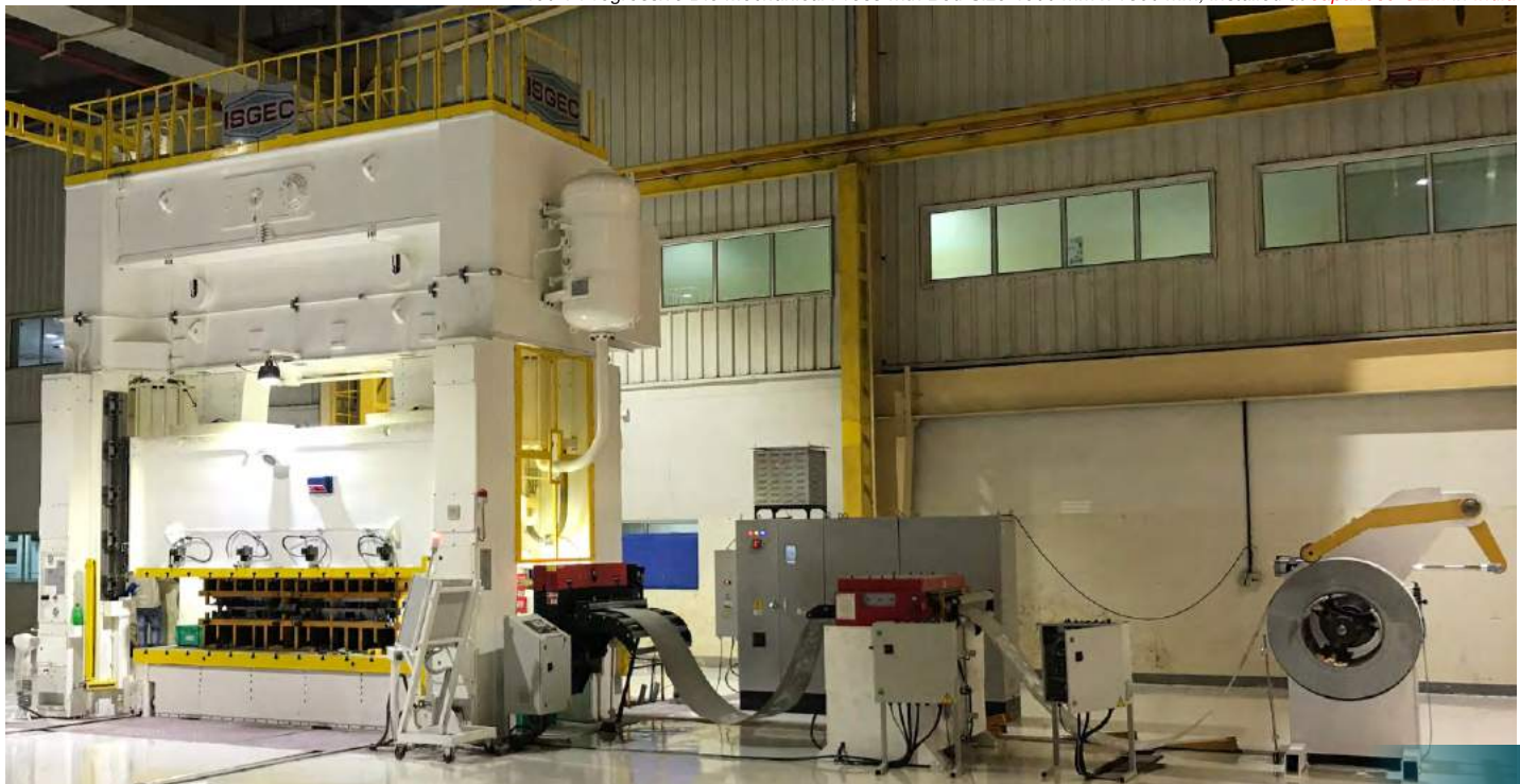
400 T Progressive Die Mechanical Press with Bed Size 4000 mm x 1500 mm, installed at Japanese OEM in India
