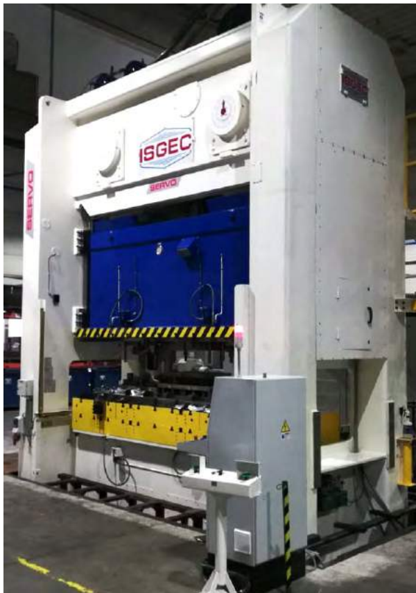
630T & 400T Straight Sided Servo Mechanical Press supplied to a customer in Hungary
