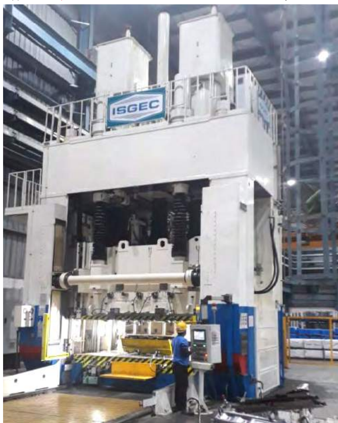
1200 T Tryout cum 300 T Die Spotting Press with 180 deg Slide Tilting feature supplied to Japanese Auto Tier-1 for their JV in India for Suzuki Project
