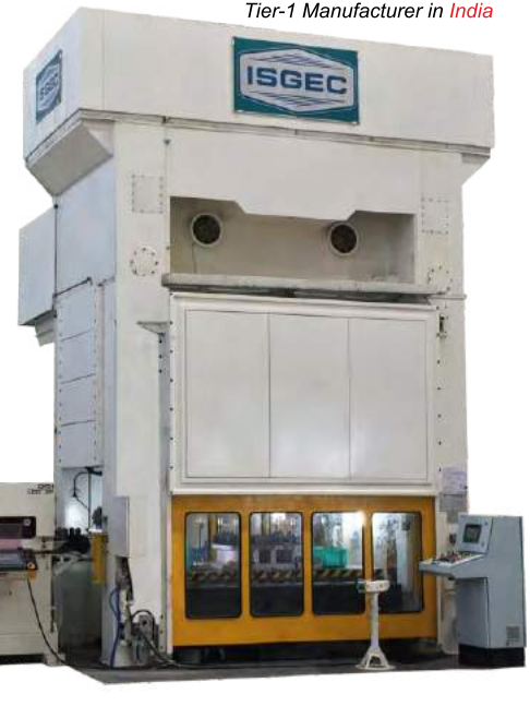
400 T Progressive Die Mechanical Press with Bed Size 4000 mm x 1500 mm, installed at Japanese OEM in India
