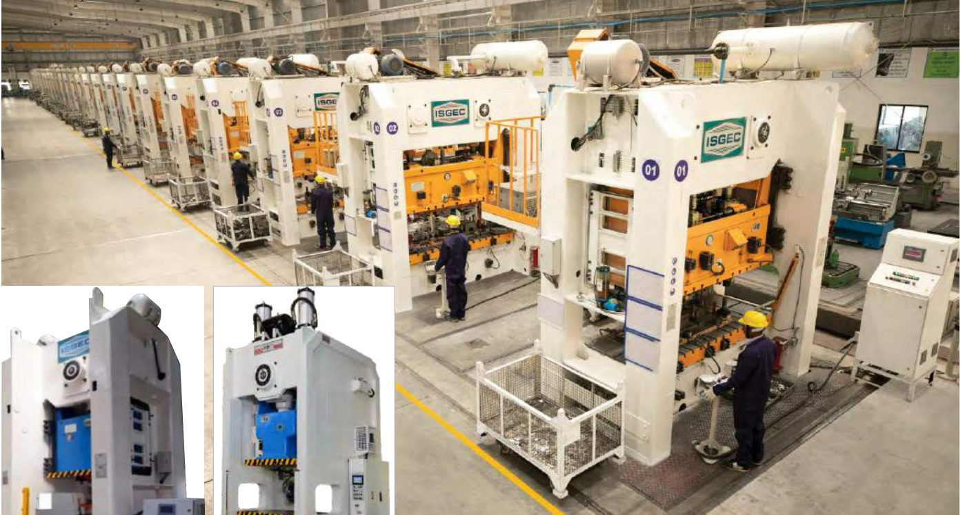
Battery of MAX 2 Series Monolithic Frame Double Crank Presses ranging from 200 T to 400 T capacity supplied for Progressive & Stamping Applications for Two Wheeler Components to Auto Tier-1 in India. MAX 2 Models are available from 200 T to 630 T
