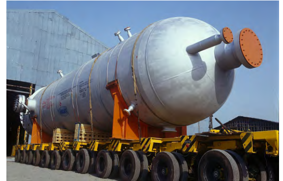
Isgec supplied this High Pressure Separator Vessel to SNC Lavalin, Canada. This Vessel, having Stainless Steel weld overlay was used in a Gas Processing Plant that they built for Petroleum Development Oman. The vessel weighs 210 Tonnes.
