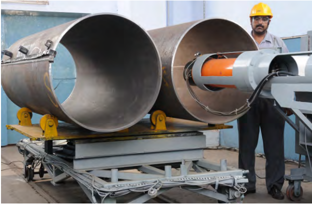
Such X-Rays further prove that all welds are sound
