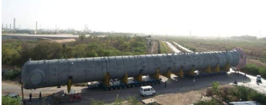
880 MT, 92 M Long, C2 Splitter Column for Customer in Mexico
