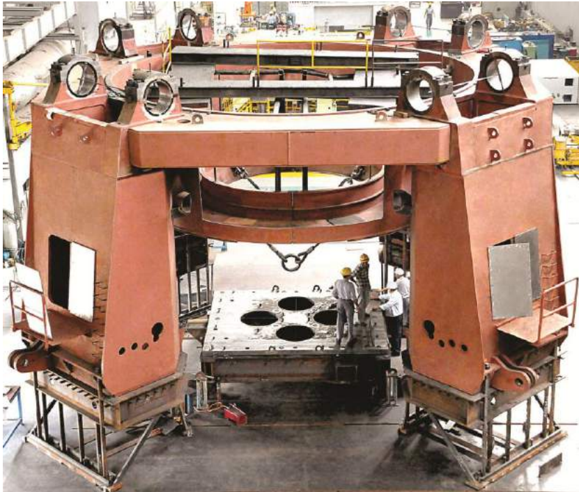
Cement Mill Stands Design : Loesche, Germany
