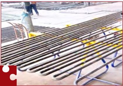
SEL Manufacturing Co. Ltd.: Supply of Bed Superheater Coil Bends and Economiser Coil for Cethar Boiler
