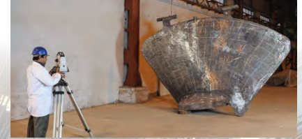
Profile measuring using Theodolite System
