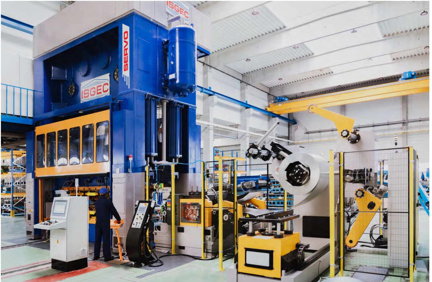
630MT Progressive Die Servo Mechanical Press equipped with Mechanically & Electrically Synchronized Multi-Servo Motor installed with a Spanish MNC for their plant in Nitra, Slovakia
