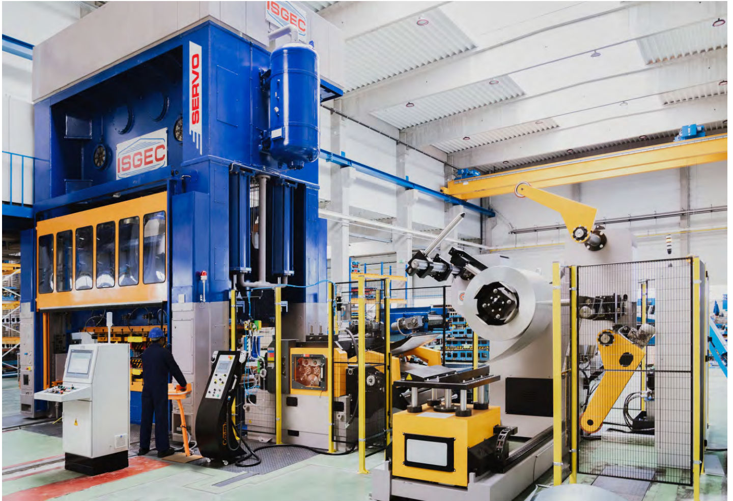
630MT Progressive Die Servo Mechanical Press equipped with Mechanically & Electrically Synchronized Multi-Servo Motor installed with a Spanish MNC for their plant in Nitra, Slovakia
