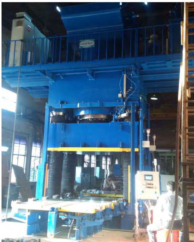
3000 T Servo Hydraulic Press With Charge Filling Automation
