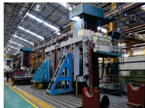
Horizontal Boring Machines
