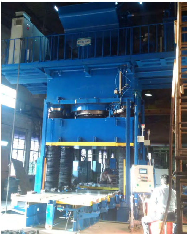
3000 T Servo Hydraulic Press With Charge Filling Automation
