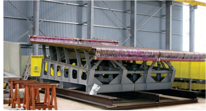
Fourth Generation Water Cooled Gate
