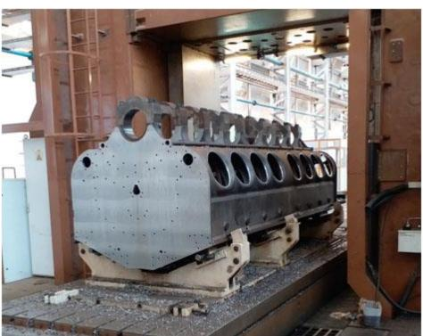
Fabricated & Machined Diesel Engine Block for Railways
