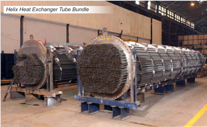
High Pressure Ammonia Synthesis Loop Heat Exchanger for a Fertilizer Plant, India
