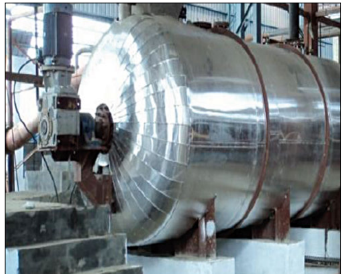
Figure 4. Continuous type horizontal sugar melter
