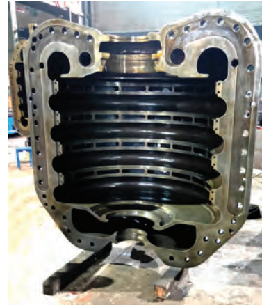
Casting of Housing for a Rotary Ammonia Compressor supplied to a Process Plant in Russia
