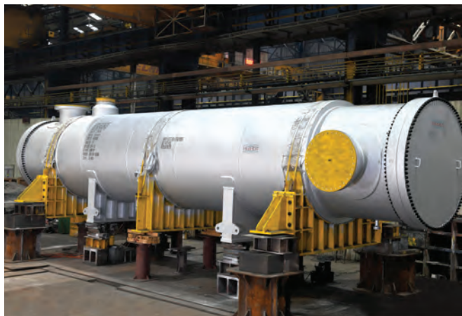
High Pressure Heat Exchanger supplied to an Ammonia Plant in USA
