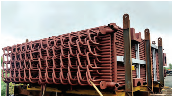
Super Heater Module supplied to a Waste to Energy Plant in Australia
