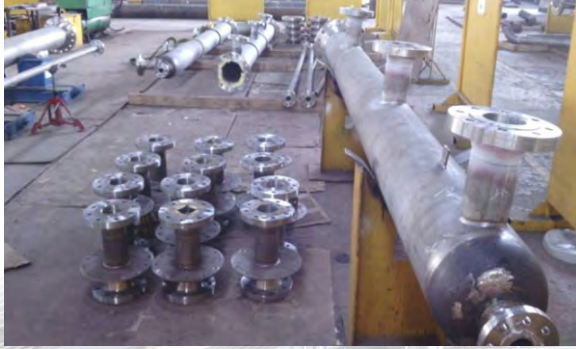
Compressor Piping Spools
