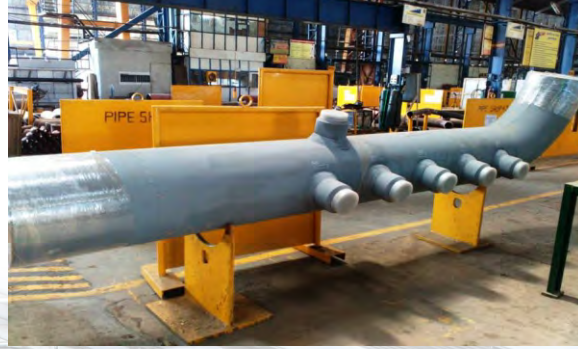
Pre-Fabricated Piping Spool
