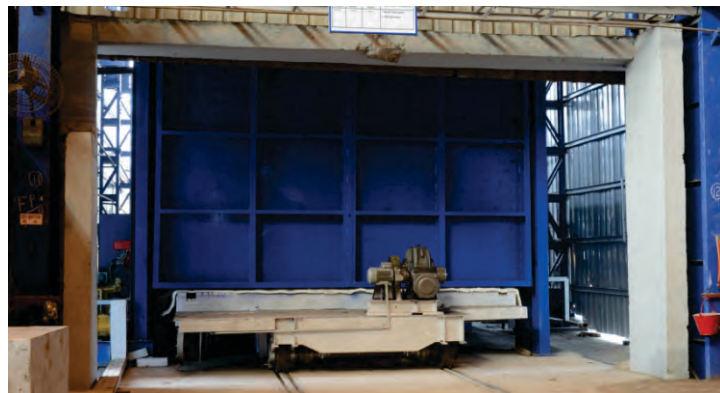
Heat Treatment Furnace (Size up to 23 M X 3.5 M X 4M)
