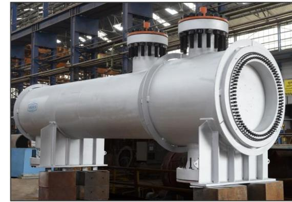
Breech Lock Closure Type Heat Exchanger for a Refinery in India
