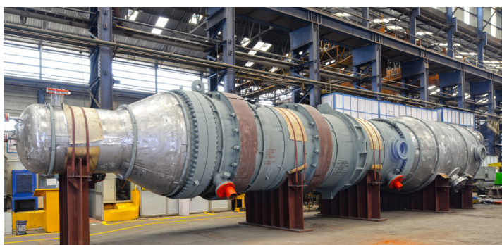
Medium Pressure Decomposer with three tube sheets for a urea plant.
