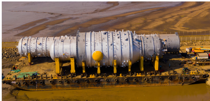
Large Vacuum Distillation Column of diameter more than 13 m weighing close to 1,000 MT supplied to Thailand.
