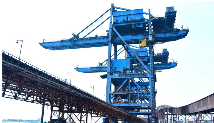
Ship Unloaders supplied to a port in eastern coast of India with a capacity of 2,750 TPH and a height of 60 m.
