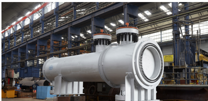
Breech Lock Heat Exchanger for hydro processing units of oil refinery with tube side pressure up to 199 bar.
