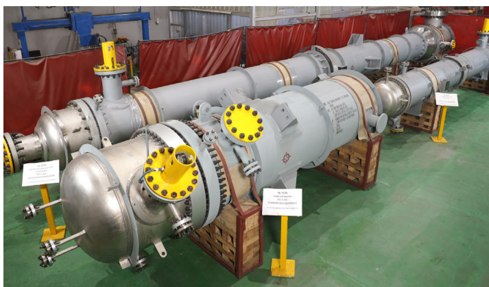
Titanium Exchangers for purified terephthalic acid (PTA) plant.
