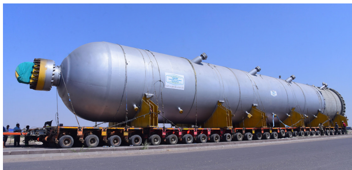
Vanadium Alloy Steel Reactor for hydroprocessing unit.
