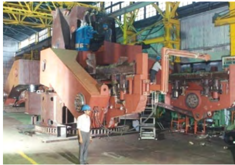
Ladles Turret for Steel Melting Shop (SMS)
