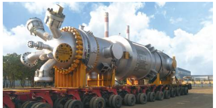
Reform Gas Waste Heat Boiler
