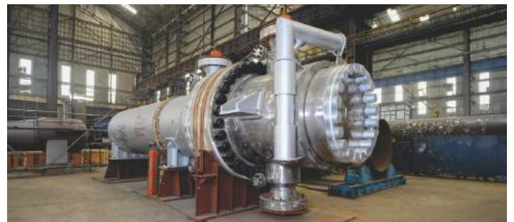
HP Heat Exchanger
