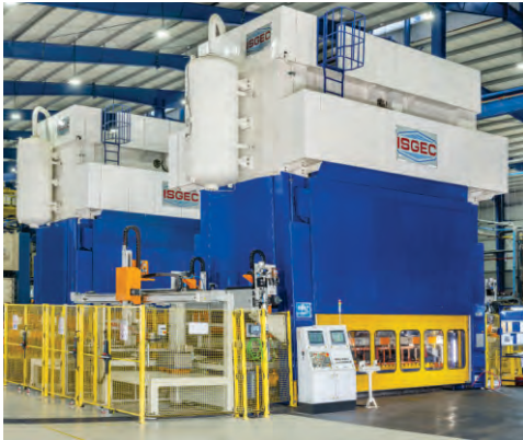
10000kN & 10000kN Transfer press with Bolster size 5000mm x 1500mm
