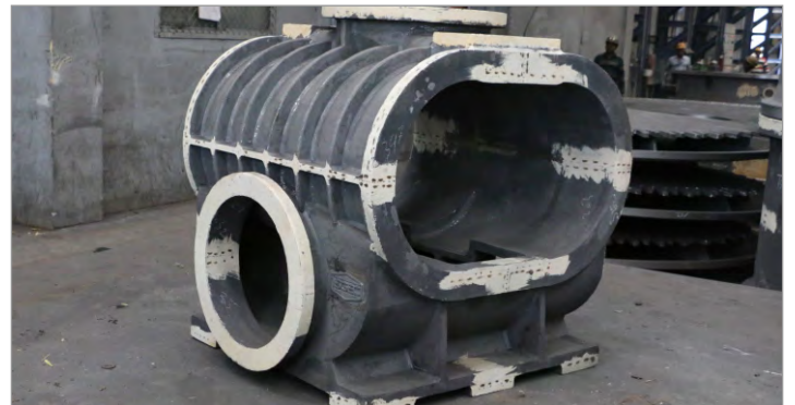
Casing Casting for Blower
