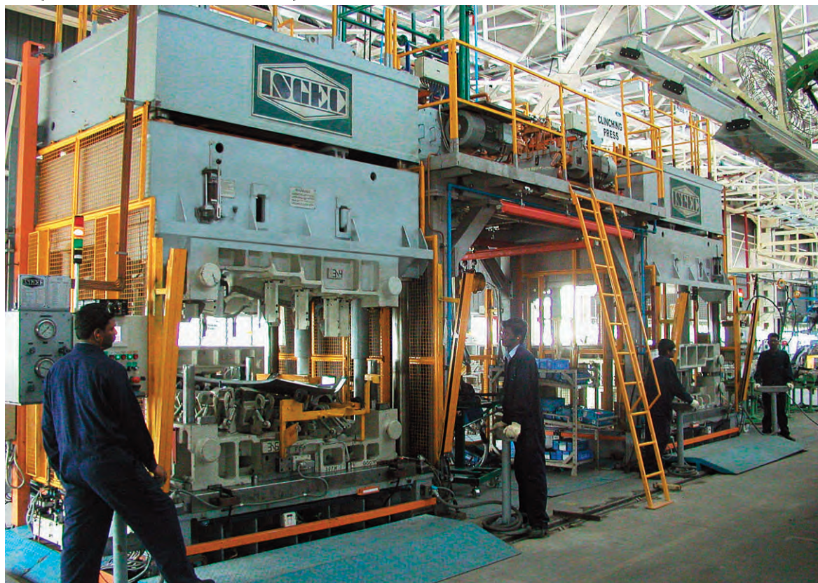
Isgec has supplied Hemming Presses to Maruti Suzuki, Ford India & Honda Cars . The Presses in the picture, installed at Ford India, are equipped with Die Carts and a Die Parking System for fast & efficient changeover.
