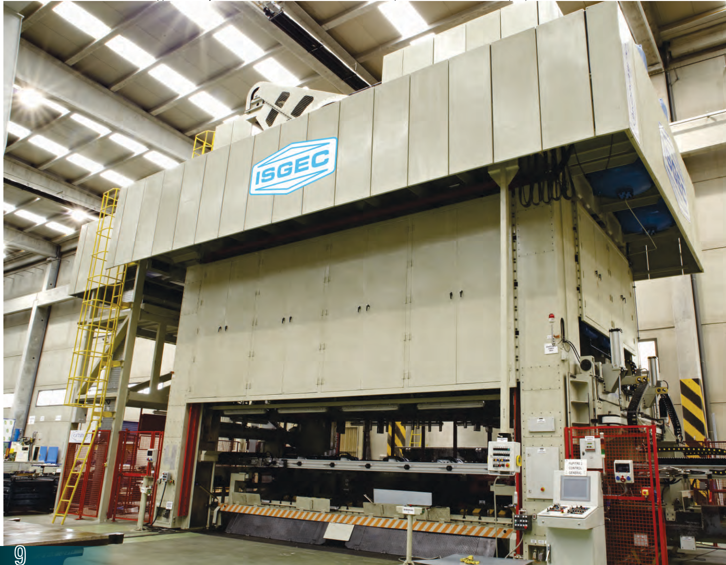
25000 kN Transfer Press supplied to CIE Automotive, Egana, Bilbao, Spain, with Bolster size 7000 mm x 2750 mm, 3-Axis Electronic Servo Transfer System and Coil Feed Line. The Press was supplied in the year 2009 and is used for manufacture of components for General Motors (GM).
