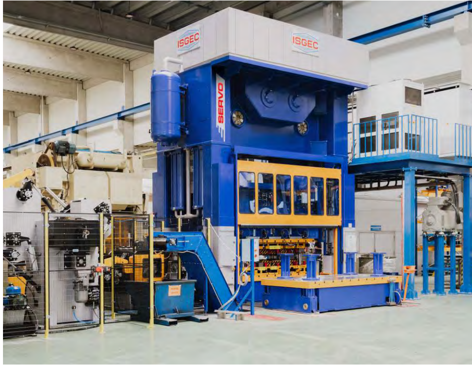
630T Servo Mechanical Press with Bolster Size 3400 x 1600 and 3-50 spm installed in Slovakia for Progressive Application
