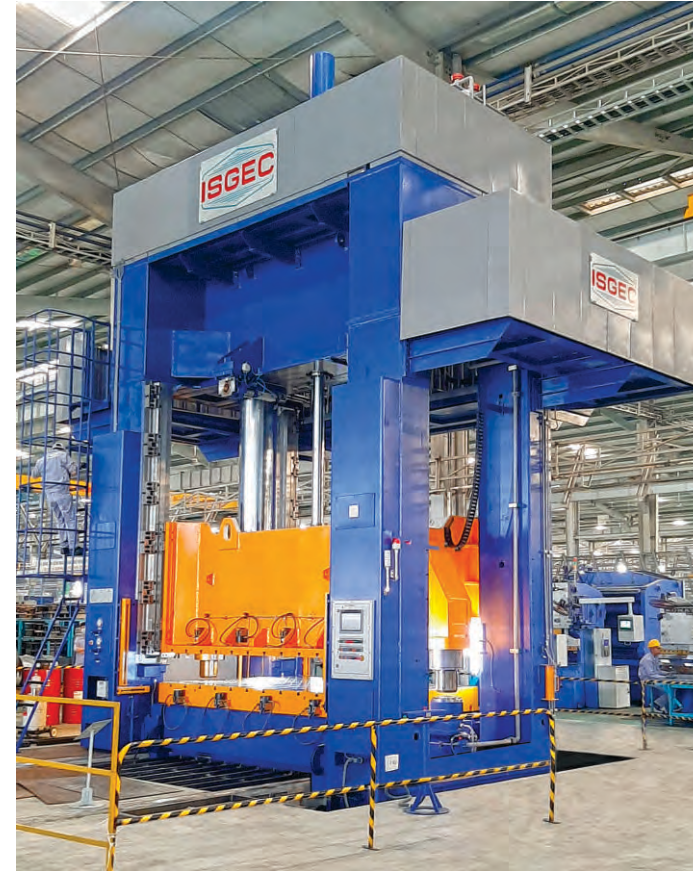
1000T Hydraulic Press supplied to an Auto OEM in Vietnam for deep draw components of commercial vehicles
