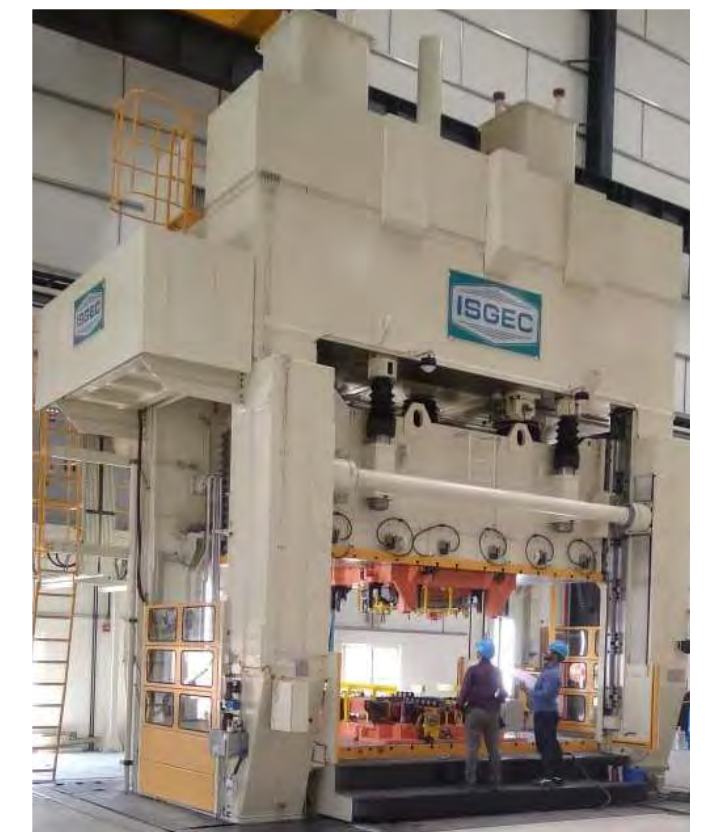
1000T Tryout cum 300T Die Spotting Press supplied to Japanese Stamping Dies manufacturer in India
