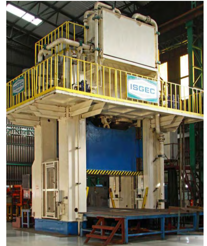
2400T Hydraulic Press supplied for manufacturing of Hot Forming Application of Axles to Automotive Tier-1 Industries
