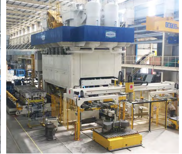
2500T Transfer Press with Bolster size of 6100 x 2500 integrated with European make 3-axis Servo Transfer system supplied to Auto Tier-1, India for manufacturing components to Suzuki
