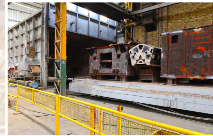
Stress Relieving Furnace
