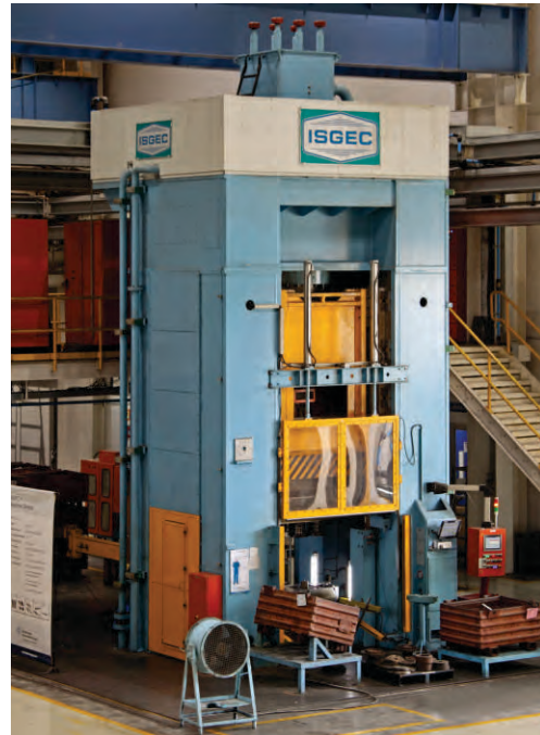
16000 kN Hydraulic Press supplied to Hirschvogel Group for their plant in Pune, India. This press is being used to manufacture cold forged transmission components used in Automotives.
