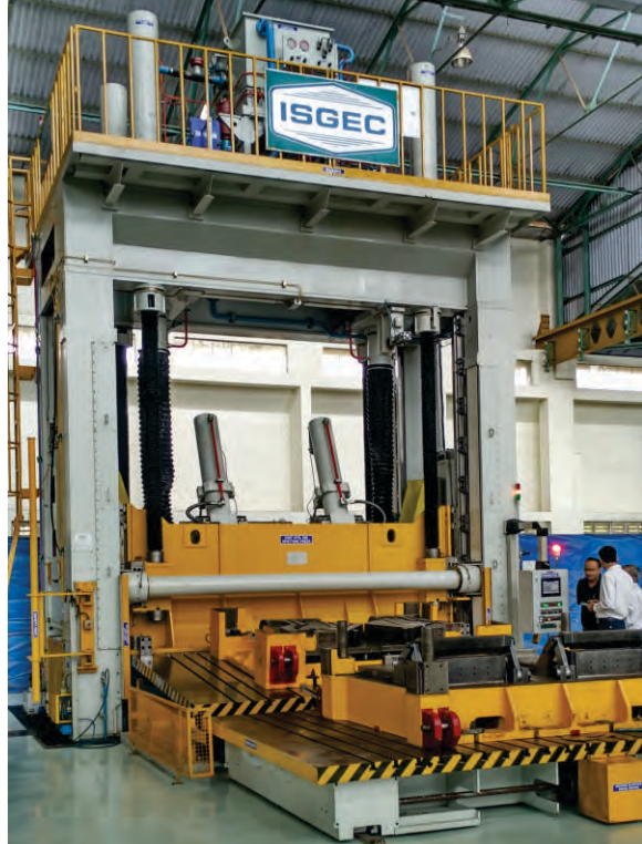
2000 kN Die Spotting Hydraulic Press supplied to Bajaj Auto . This Press is equipped with feature of 180 Deg Reversal of Top Die to carry out corrections in top die safely
