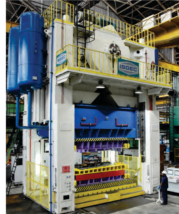
20000 kN Mechanical Tryout Presses with full force Micro Inching supplied to Tata Motors
