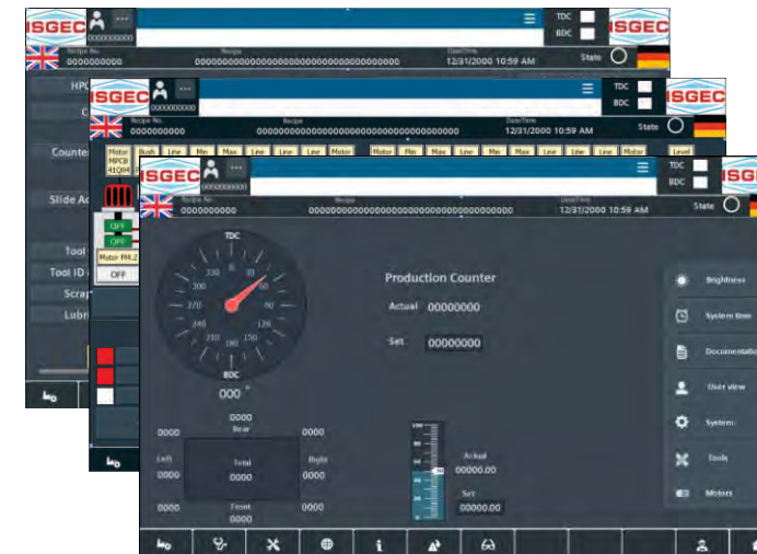
Dedicated software has been developed by Isgec for Press System Controls. The user friendly software is used for instant diagnostics. This picture is of the Main Menu Touch Screen.
