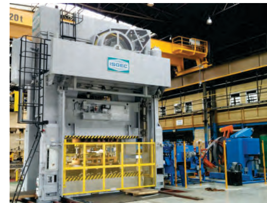
6300 kN Progressive Die Mechanical Press supplied to Comaco Group for their plant in Poland. The press has a bed size of 3700 x 1600 mm, Slide Stroke 400 mm and speed of 22-44 spm. Identical presses supplied for their plants in Mexico and Brazil.
