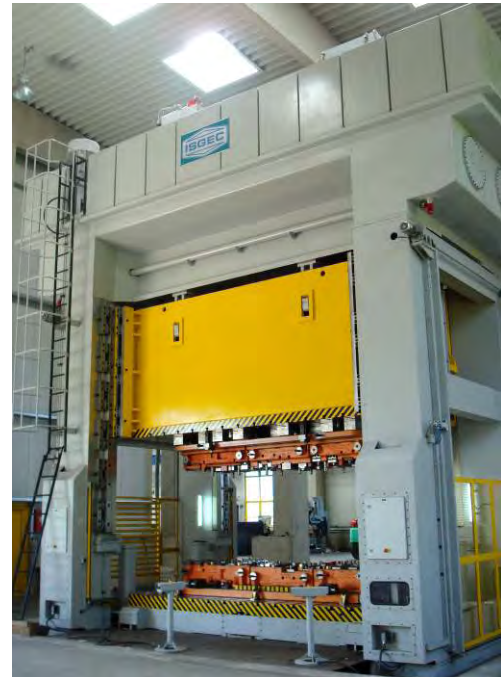
This 12000 kN Hydraulic Press was supplied to UTW, at Drolshagen-Scheda, Germany for tryout and manufacturing critical components for Auto majors. The Press is equipped with moving bolster of size of 4500 mm x 2200 mm and has provision for mounting Dampers, which makes it suitable for blanking.
