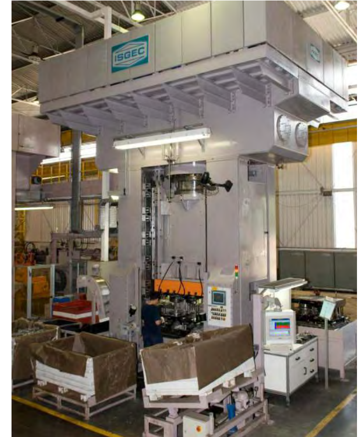
1500T Hi-speed Hydraulic Press supplied to a German MNC in Brazil for manufacturing Clutch Components. Similar supplies made to their plant in South Africa & India
