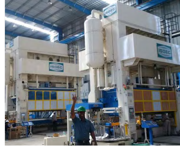
1250T with Bolster Size of 4300 x 1400 & 630T with Bolster Size of 3700 x 1400 integrated with Korean make transfer system supplied to Auto Tier-1, Bangalore, India supplying majority to most 4 Wheeler & 2 Wheeler OEM's
