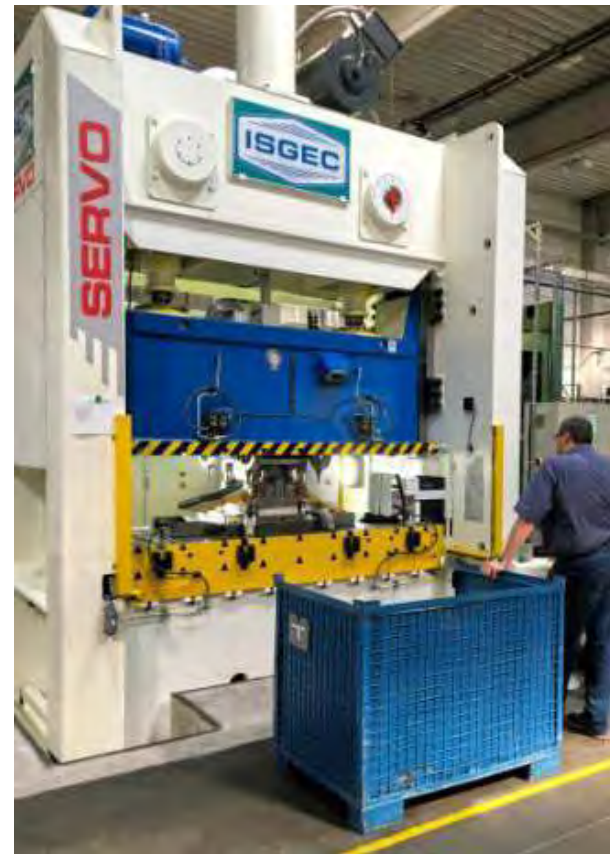
400T Straight Sided Frame Servo Mechanical Press supplied to Hungary
