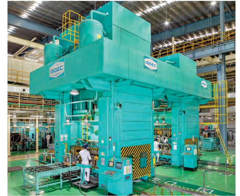
630T Link Drive & 400T Eccentric Gear Drive Tandem Line supplied to Japanese OEM in India for manufacturing of Two Wheeler Components
